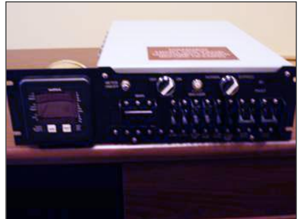
Power Distribution Unit Control Panel
